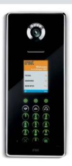
Digital push-button panel with IP protocol and soft-touch panel. Features 3.5" colour display, alphanumeric control panel, arrow keys for name index book browsing, colour camera with lighting, audio module and proximity key reader.
