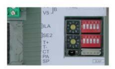
The dip-switches fitted in each device immediately associate addresses to individual users.
